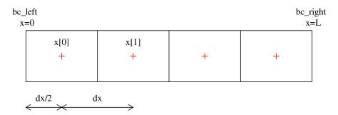
The left boundary is defined on x = 0 while the center of the first cell - which are the points constituting the finite difference nodes - is in x = dx/2, with dx = L/n.
